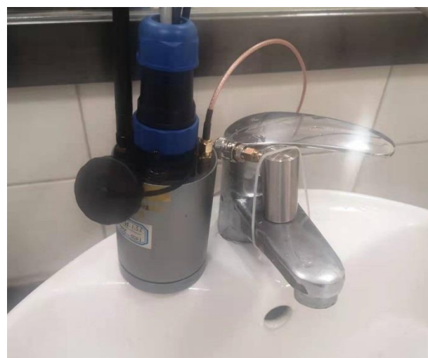
Fig. 12: Online water pipe quantitative leakage experiment system.
