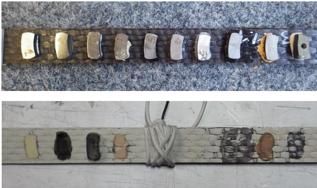
Fig. 5: top: Photo of metal plates glued to CMC before test in the oven; bottom: photo of metal plates glued to the CMC after test in the oven
