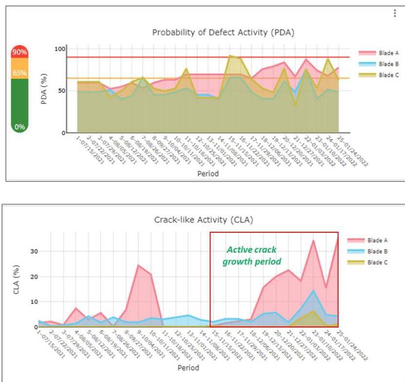
Fig. 7: PDA (top) and CLA (bottom) of a wind turbine between inspection cycles. Blade A shows high values of CLA, and inspection corroborated the appearance of a chord crack on the blade around 40m from the root.
