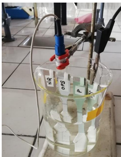
Fig. 3: Set up for pre-corrosion in a corrosive NaCl 3.5 wt % bath.
